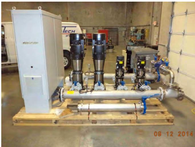
also included a Cummings standby generator for emergency power. In addition PumpTech supplied a temporary bypass booster pumping system to supply water pressure during installation of the building.
