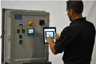
PumpTech partnered with the city of Scappoose, OR as the beta test site for iRover. In December of 2010 PumpTech installed a Hydronix 421 packaged lift station that was designed to provide continuous variable flow to a new filtering station. All that was required to upgrade the system was the installation of an Ethernet card in the
