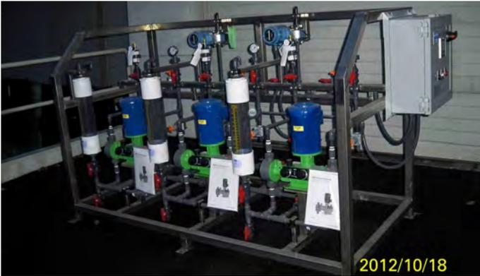
manufacturing process. This particular process required a reliable, non-metallic pump end with smooth, non-pulsing flow so Grundfos DMH dual diaphragm pumps were selected for the application. Pulsation dampeners were also incorporated to assure even smoother flow. Two pumps provide flow to two locations on the paper machine while the third
