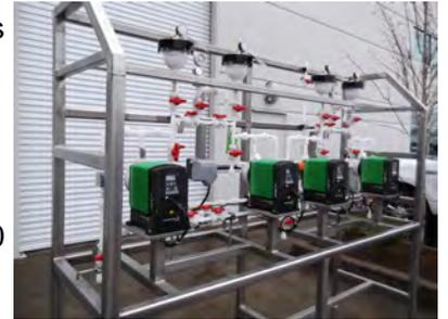
All of the piping was covered with aluminum heat transfer tape and then a 120 VAC, heat trace cable was installed. The entire assembly was then covered with an engineered foam insulation. Finally, a white engineered coating was applied to protect the insulation from moisture and UV rays. The pictures below shows a skid during insulation installation and the finished skid after coating.
